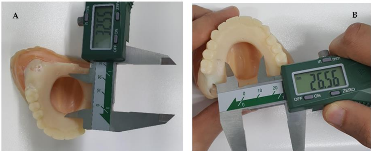
Figure 8. Digital micro caliper used to measure (A) the AP distance and (B) the lateral distance.
