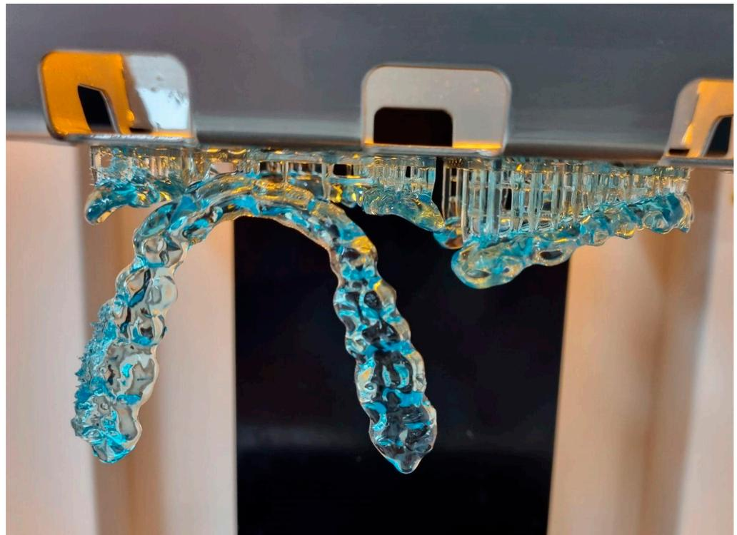
**Figure 5.** Printed splints in 0°, 30° and 90° orientations (Nextdent 5100).
