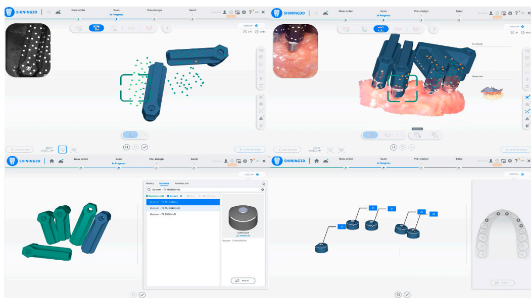
Figure 3. Elite IPG utilizing a coded pattern to calculate each scan body position in relation to the others.
