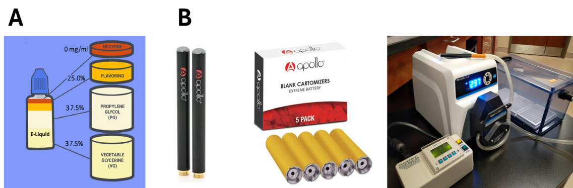
Figure 1. Description of E-liquid and apparatus. The E-liquid (A) and apparatus (B) used to expose streptococcal bacteria to E-cigarette-generated aerosol ± flavors are shown. In (B), the (left) shows the Apollo ECIG batteries; the (middle) shows the Apollo blank cartridges; the (right) shows the peristaltic pump, Traceable™ controller, and exposure chamber. Note the Tygon S3® tubing running from the E-cigarette to the pump and finally to the exposure chamber.
