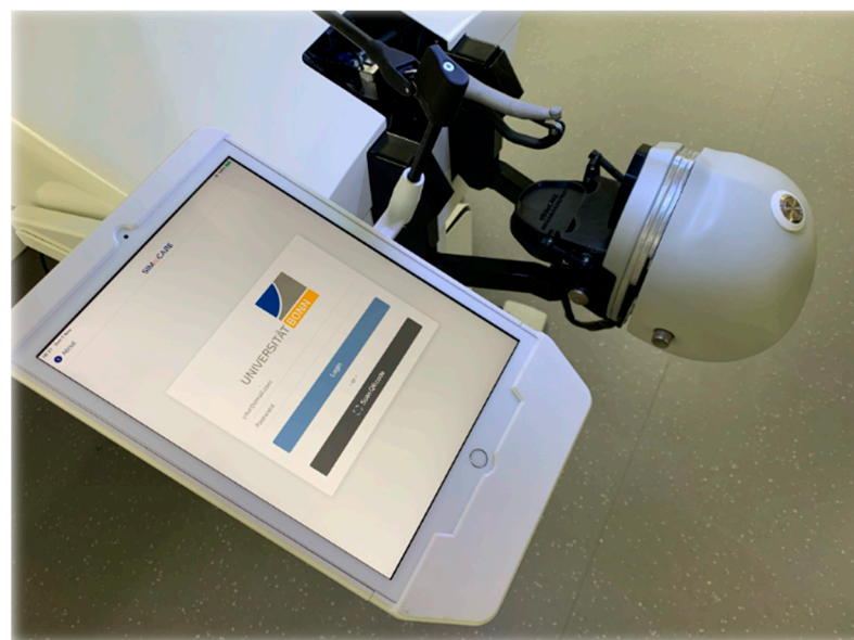
Figure 2. “Dente” simulator by SIMtoCARE (Vreeland, The Netherlands) with tablet, phantom head, and handpiece.
