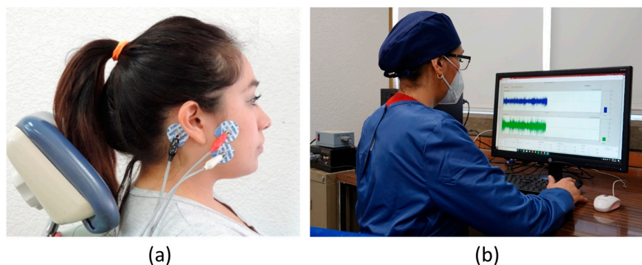
Figure 1. Electromyographic recording. (a) Placement of surface electrodes over the origin and insertion of the masseter muscles; (b) electromyographic recording in maximum voluntary contraction for 30 s, with Electromyograph 1.2 UNAM-CINVESTAV ® .
