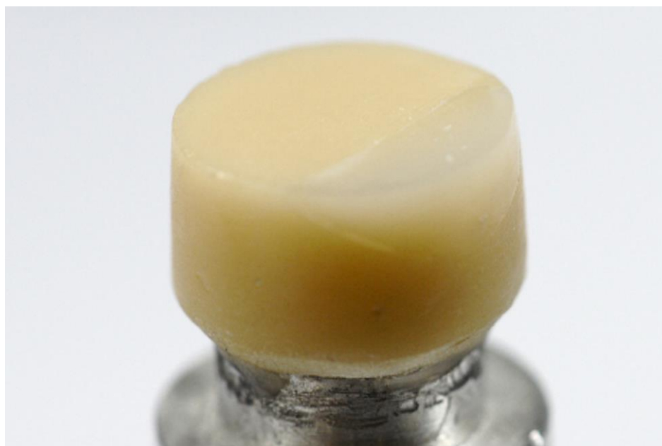
Figure 4. Repaired specimen with bonded ceramic.
