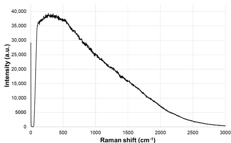
Figure 2. Spectra obtained for an Iberian ham sample, dominated by the fluorescence profile.
