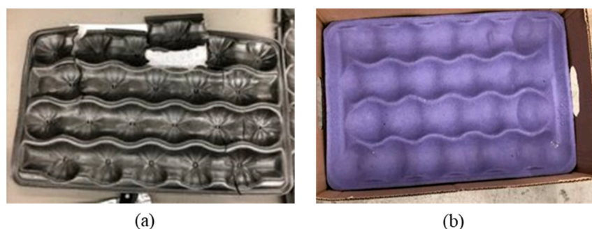
Figure 11. Example of tray damage, (a) EPS and (b) MF.
