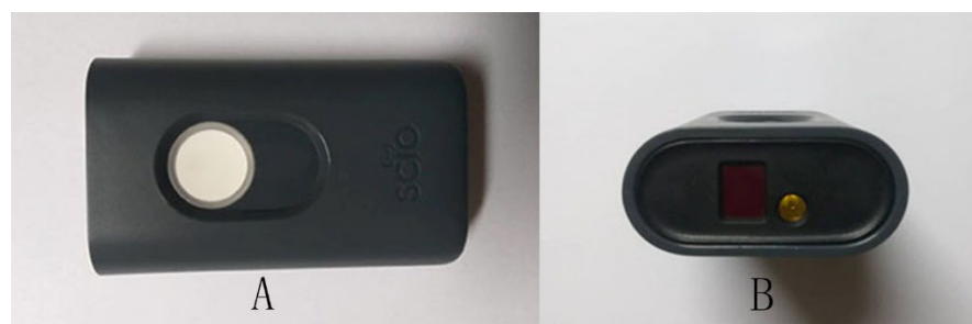
Figure 1. Consumer Physics VIS/SW-NIR molecular sensor, SCiO™ (A) VIS/SW-NIR spectrometer, (B) The location of light source and detector).
