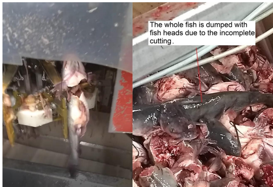
Figure 6. The waste due to deheading processes.
