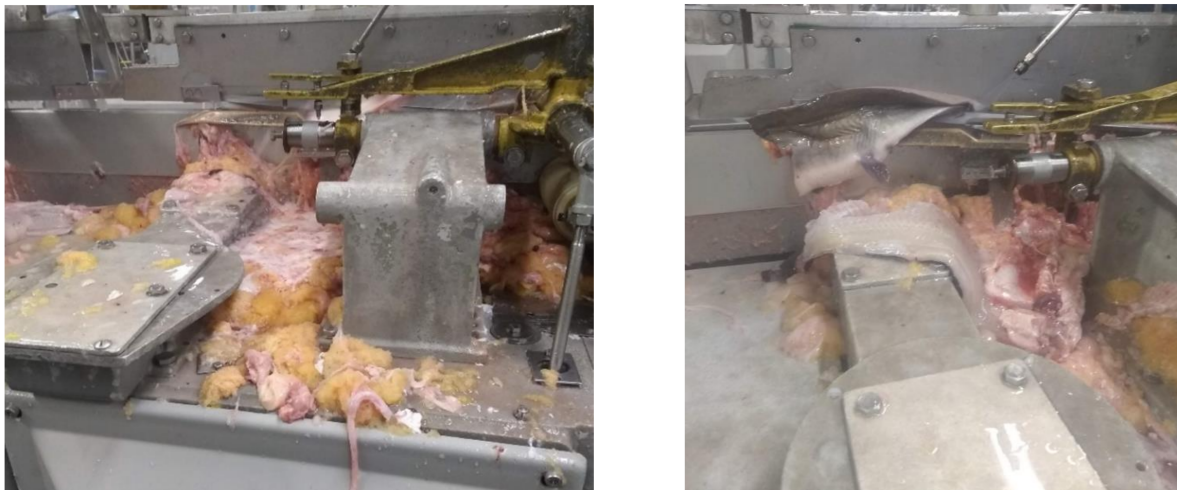
Figure 3. The filleting machine is frequently jammed because the fish guts are left in the machine. The normal filleting processing is affected by the jamming issue, which makes some fillets drop out of the machine as waste.
