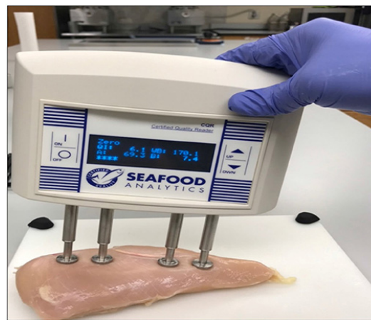
Figure 2. Hand-held BIA setup for the classification of fillets based on different myopathic conditions.
