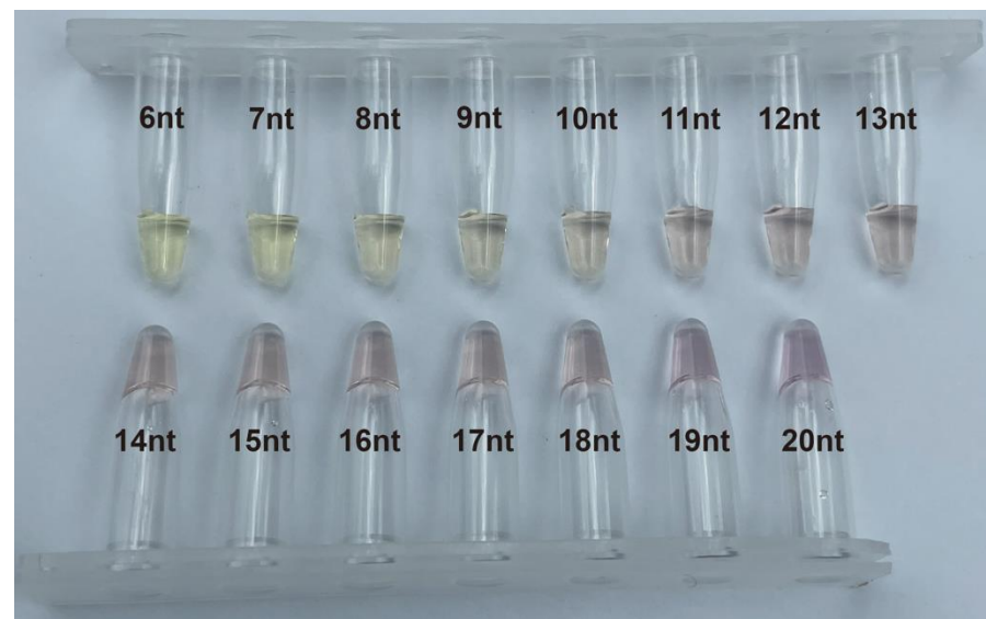
Figure 1. Color of mixed solution (PMNT with various lengths of ssDNA).
