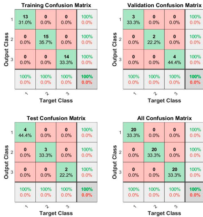
Figure 6. Confusion matrix for lemon classification (outputs: 1: Category “extra”, 2: Category I, 3: Category II).
