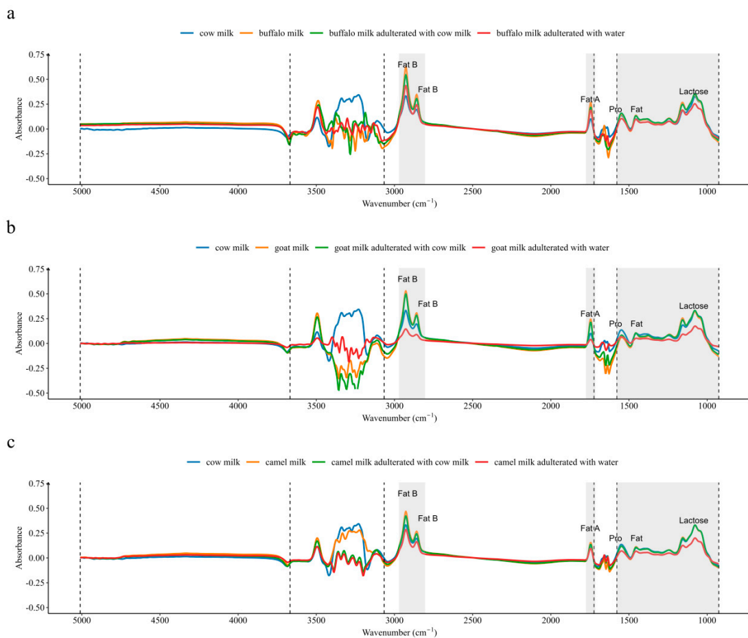
Figure 1. Original mid-infrared spectroscopy. (a) Buffalo milk; (b) Goat milk; (c) Camel milk. Gray shadow represents the region used for modeling.
