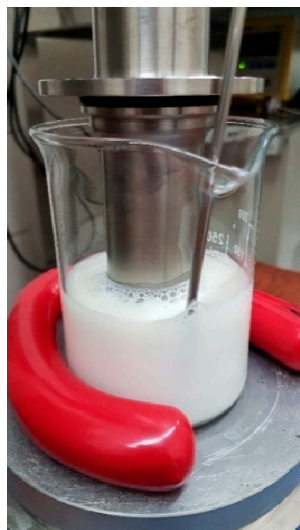
Figure 1. Batch ultrasonication of micellar casein suspensions.
