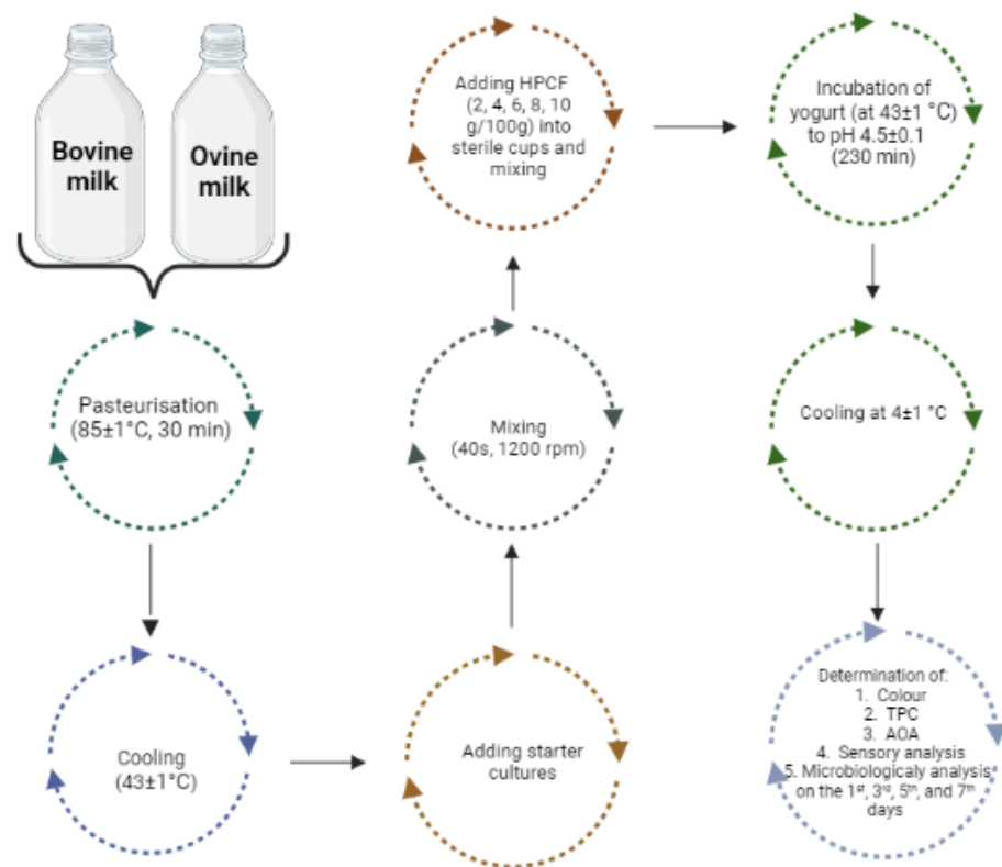
Figure 1. A schematic illustration of the yoghurt production steps (plain and fortified with hemp press cake flour) and the analysis performed on the yoghurt samples.
