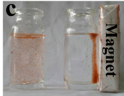
Figure 5. Photograph of magnetic microsphere particles suspended in water and under the presence of an externally placed magnet. Reprinted with permission from [39].
