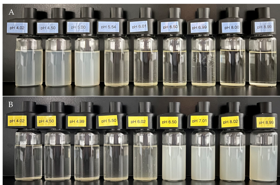
Figure 1. Appearance of zein nanoparticles prepared at pH 4.0 (A) and pH 9.0 (B) as a function of pH.
