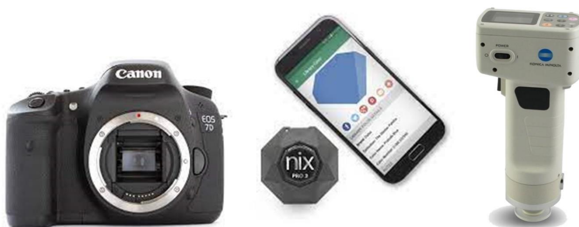
Figure S2. Colour measurement devices; Canon EOS 7D DSLR camera (left), Nix and associated smartphone app (middle), and Minolta CR400 (right).
