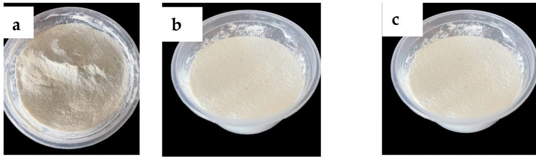
Figure 3. Hydrocolloids from (a) moringa seed, (b) egusi seed, and (c) makataan seed.
