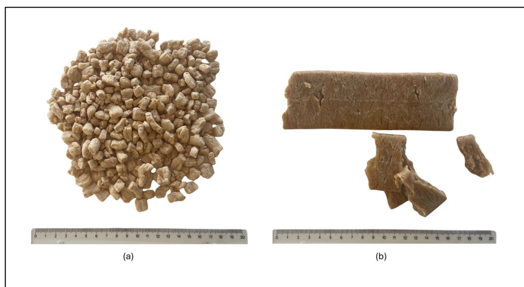
Figure 1. (a) Pea protein extrudates (TVPs) obtained by low moisture extrusion and (b) Faba bean and pea extrudates (HMMAs) obtained by high moisture extrusion.
