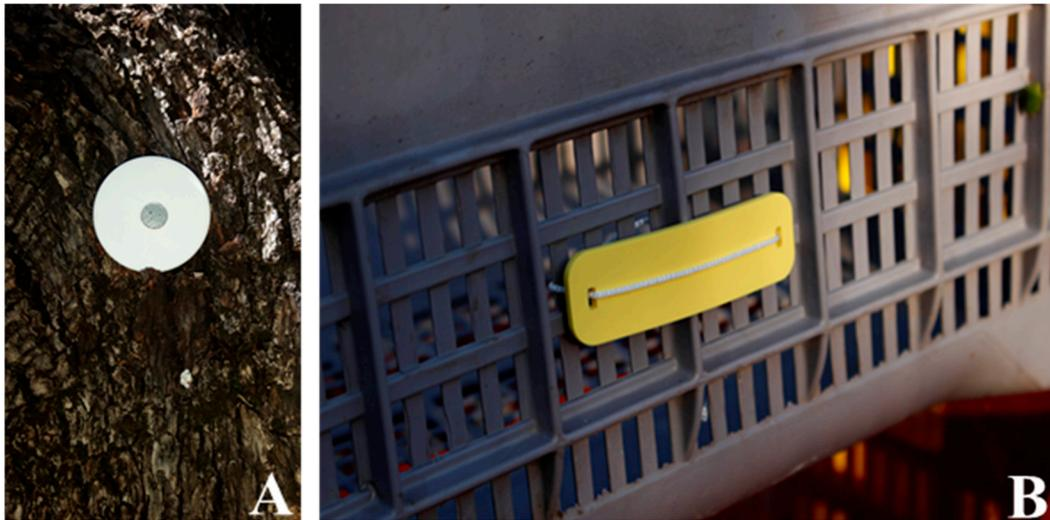
**Figure 2.** (A) The RFID1 standard used is UHF at 860 MHz, Class 1 Gen 2, waterproof coin shaped with central hole; (B) the RFID2 is UHF at 860 MHz, waterproof flexible band with two holes at the extremities fixed with a small cord on the crate.
