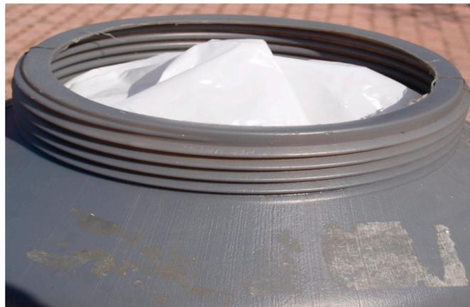
**Figure A3.** Modified industrial barrel with air-protected headspace.
