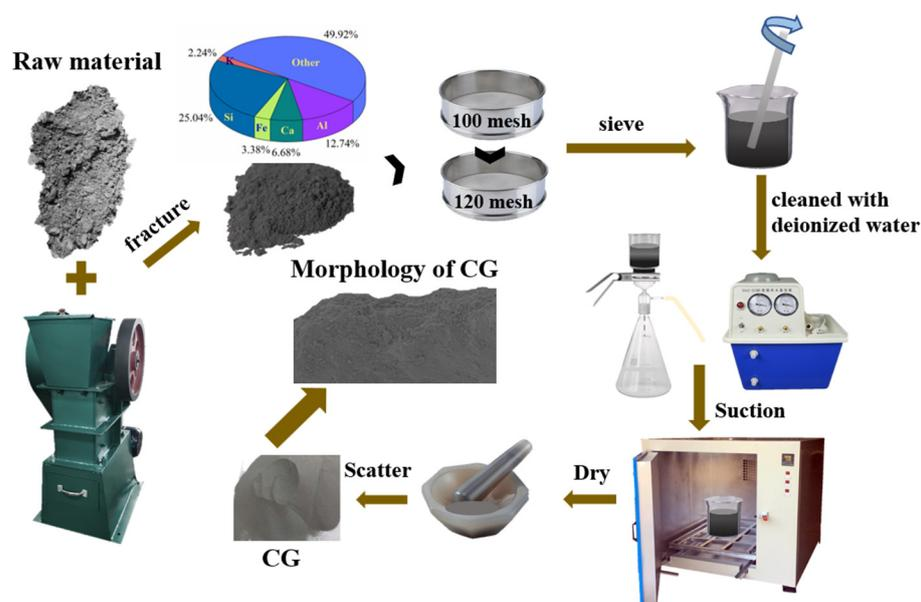
**Figure 1.** The flow chart for treatment of CG samples derived from the discarded natural coal gangue.
