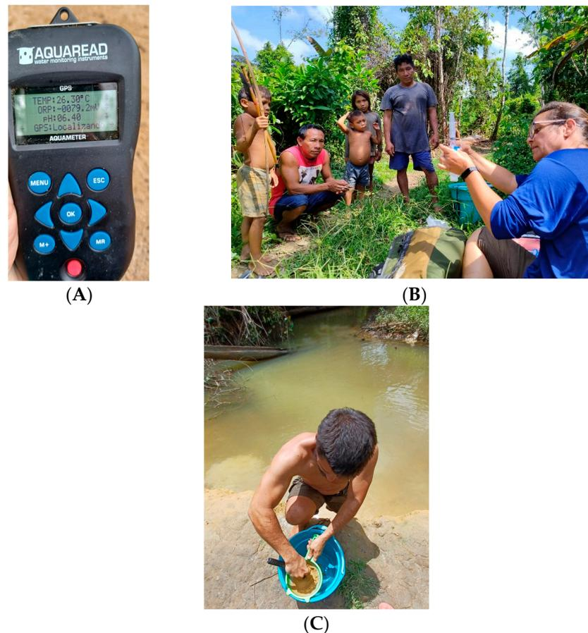
**Figure 2.** (A) Probe with some water measurements. (B) Water collection. (C) Stream sediment collection with sieving.
