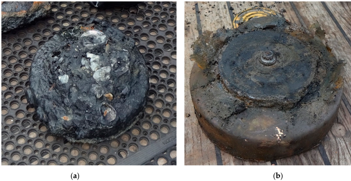
Figure 4. Images of a surfaced anti-tank mine: (a) as found on the seabed and (b) after removal of fouling.
