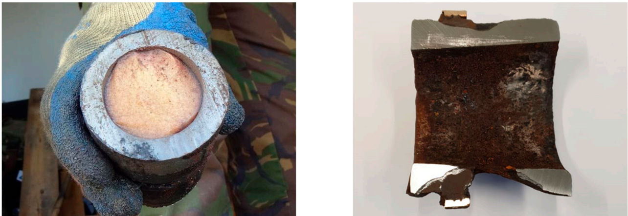
Figure 5. Cross-section of a high-explosive 75 mm recoilless rifle grenade found on the seabed, before and after removal of the energetic content.
