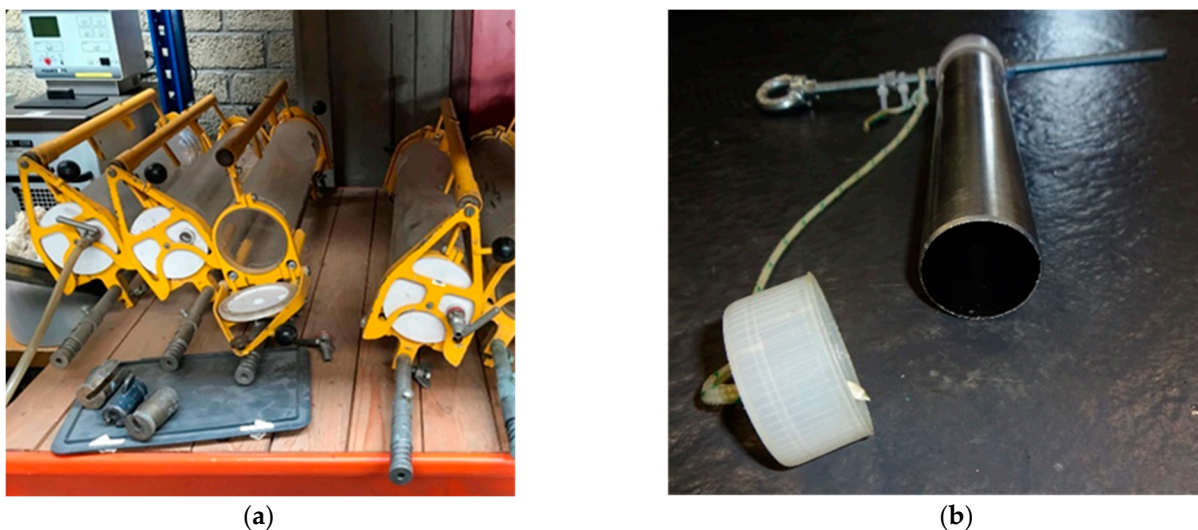
Figure 3. Tools for water and sediment sample collection: (a) water sample collection bottles with a volume of 3 L, and (b) tubes for sediment sample collection with a diameter of 40 mm. Samples for metal analysis were collected using polypropylene tubes.
