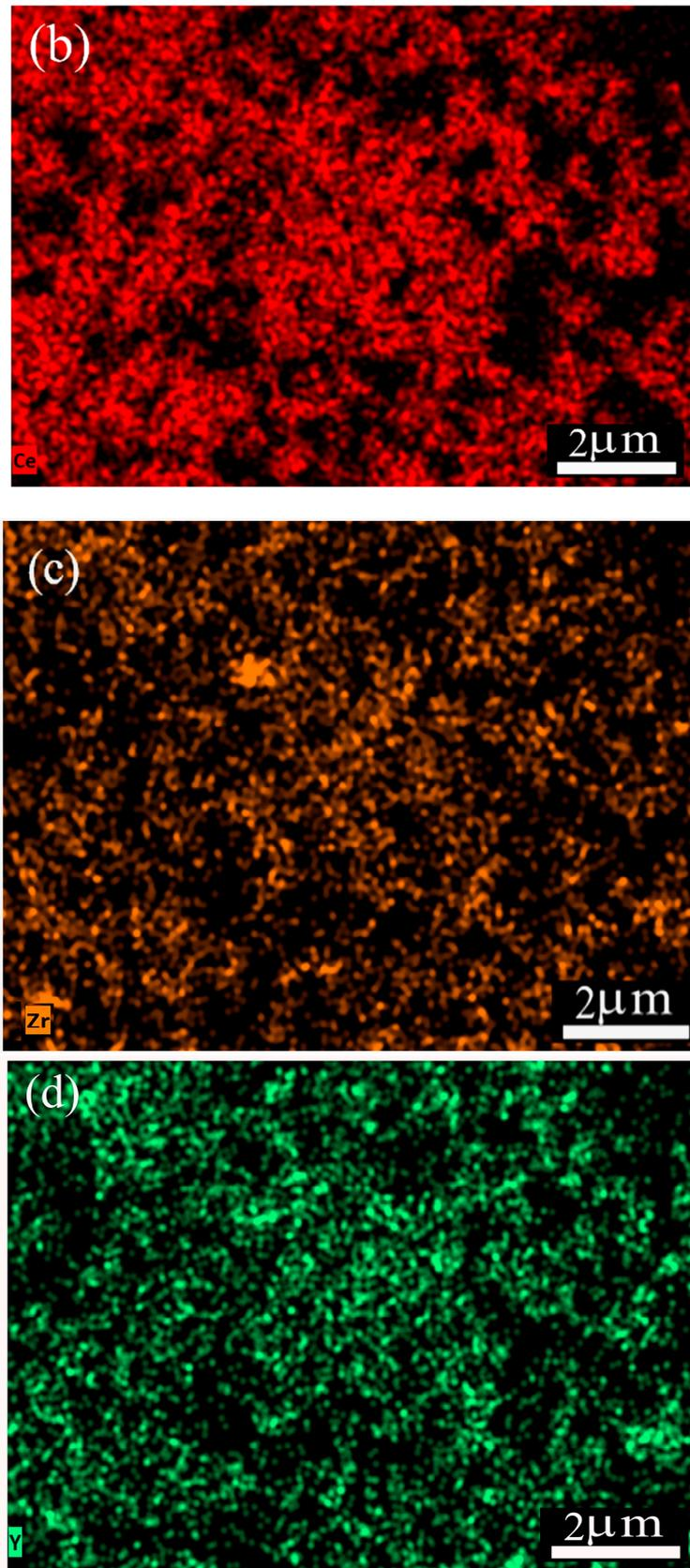
**Figure 2.** SEM images and chemical element mapping of CZY powder: (a) CZY powder obtained by milling and calcination, (b) elemental analysis of cerium, (c) zirconium, and (d) yttrium.
