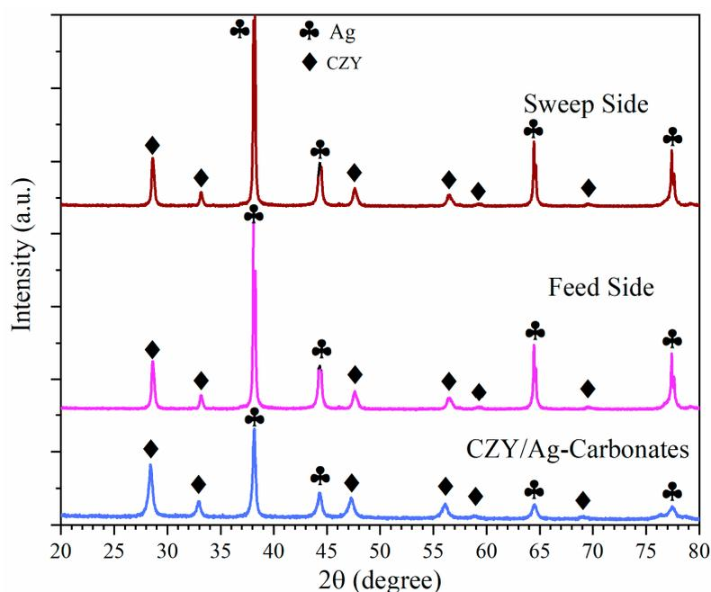
**Figure 9.** XRD pattern of the dense ceramic—carbonate membrane before testing and after continuous operation for 115 h from both the feed and sweep sides.
