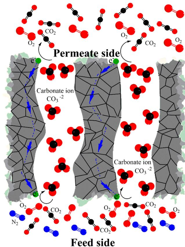
**Figure 1.** Schematic showing the selective separation of CO<sub>2</sub> and O<sub>2</sub> across a metal–carbonate membrane system at elevated temperatures.
