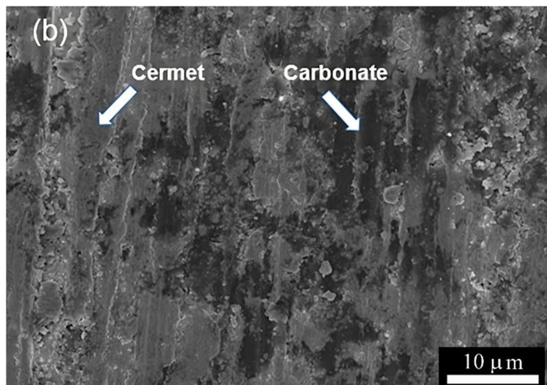
**Figure 4.** (a) SEM micrographs of porous cermet support (cross-section) without carbonate and (b) dense membrane after carbonate infiltration.
