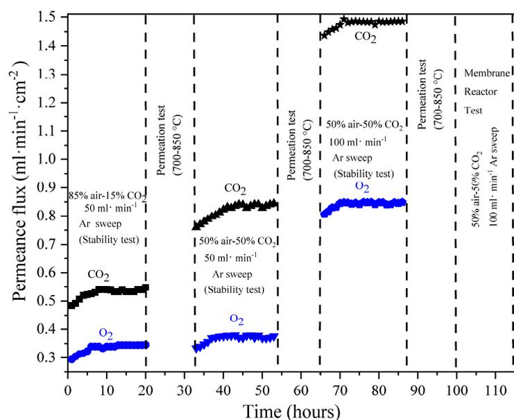
**Figure 8.** The stability performance of CO<sub>2</sub> and O<sub>2</sub> permeation at different operating conditions was studied for the dense cermet-carbonate membranes, completing a total and continuous operating time of 115 h.
