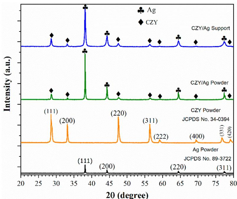
**Figure 5.** XRD diffraction patterns of silver powder, CZY powder, cermet powder, and membrane support sintered at 900 °C for 20h.
