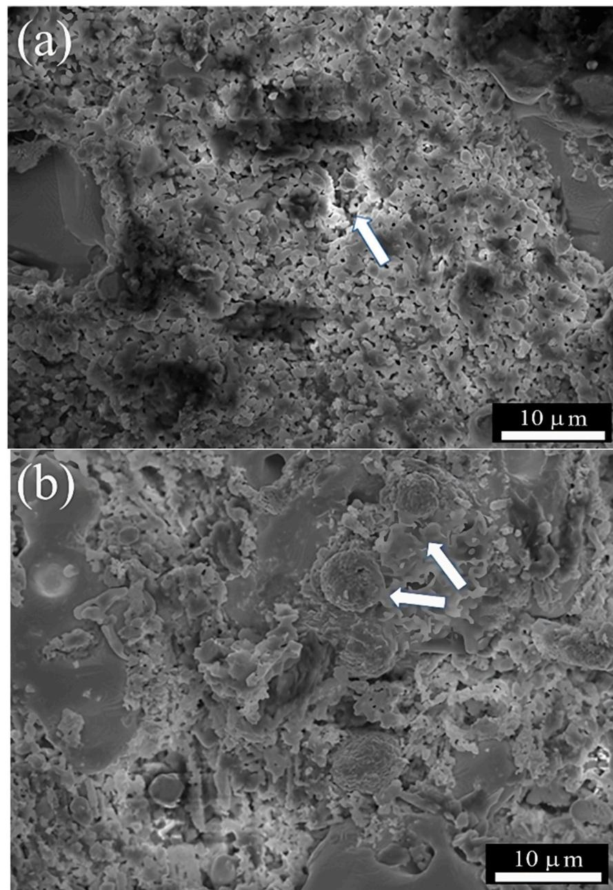
**Figure 10.** SEM images of the membrane surface after 115 h of continuous operation: (a) surface exposed to the feed gas mixture and (b) surface exposed to the permeate; with the arrows show the coarsening of Ag phase.
