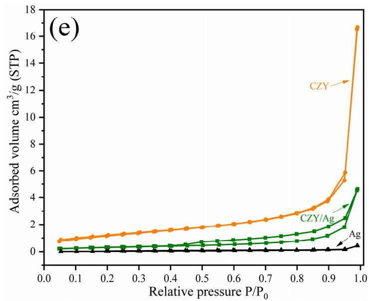
**Figure 3.** (a) SEM images of the starting silver powder, (b) CZY/Ag cermet prepared by high-energy milling, (c) particle size distribution of CZY/Ag powder (ultimate particle size), (d) EDS analysis of the cermet, and (e) N<sub>2</sub> adsorption/desorption isotherms.
