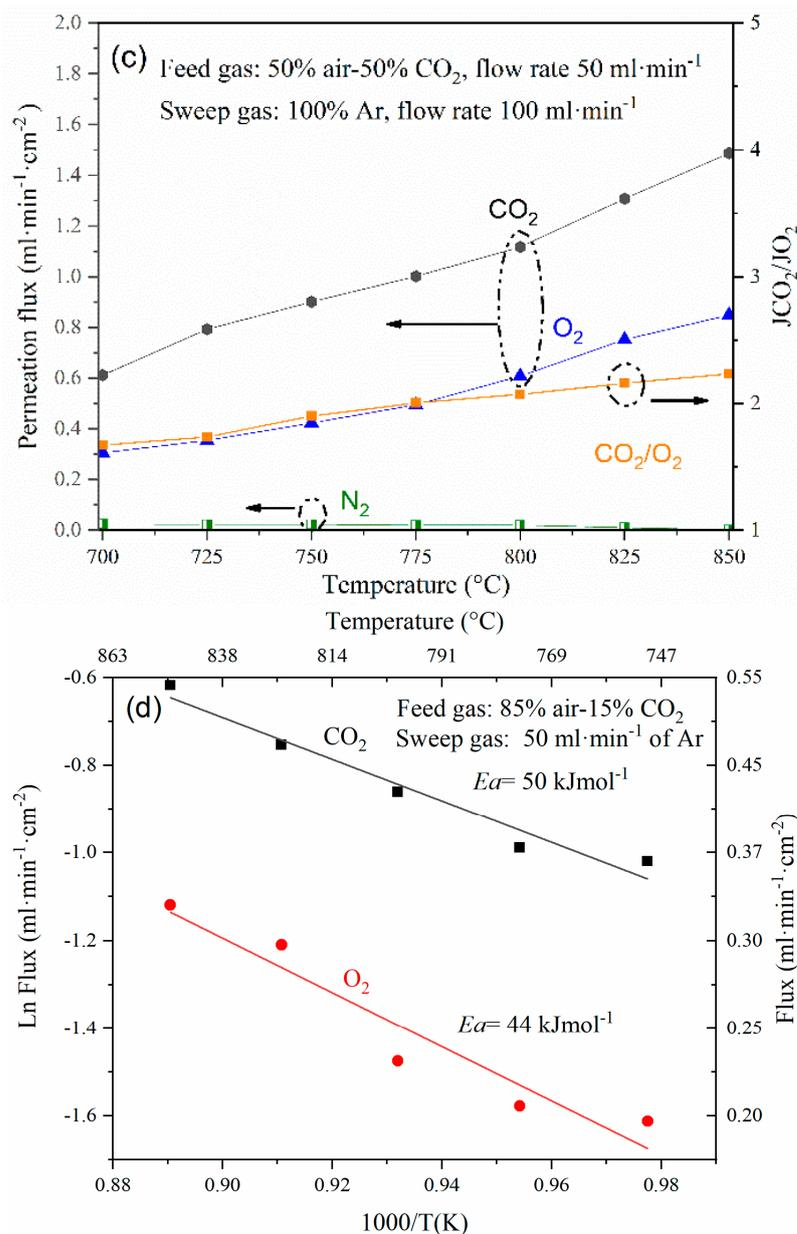
**Figure 6.** (a–c) CO<sub>2</sub> and O<sub>2</sub> permeation flux through the dense cermet membrane using different feed gas mixtures and (d) Arrhenius plot of the experiment performed with a feed of 85 vol.% air-15 vol.% CO<sub>2</sub> and sweep of 50 mL·min<sup>-1</sup> of Ar, showing its activation energy ( $E_a$ ).
