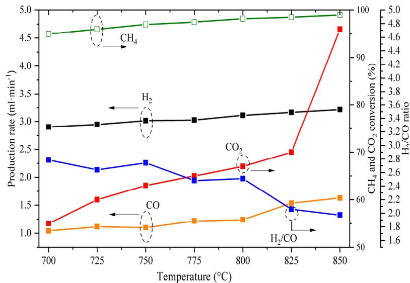
**Figure 7.** Effect of temperature on the syngas production ( $\text{H}_2 + \text{CO}$ ), methane conversion, and  $\text{H}_2/\text{CO}$  molar ratio under the studied oxy- $\text{CO}_2$  reforming of methane conditions.
