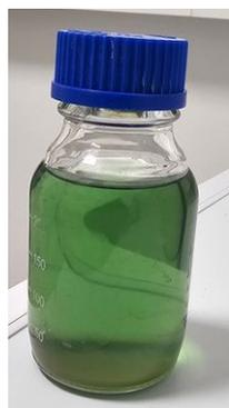
**Figure A1.** Greenish discoloration of the reaction mixture EtOH 10.00% after the reaction. The greenish discoloration shown appeared between 24 and 48 h after the photoreaction with Eu(III) was started and became more intense over time.
