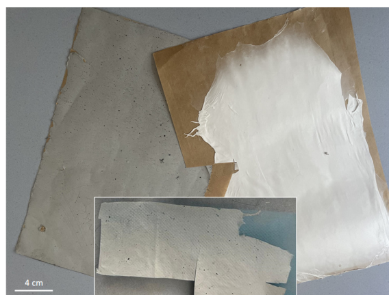
Figure 1. Optical image of electrospun fiber sheets: PVA-FLG (16%) on the left, PVA on the right, inset: PVA-FLG (4%).
