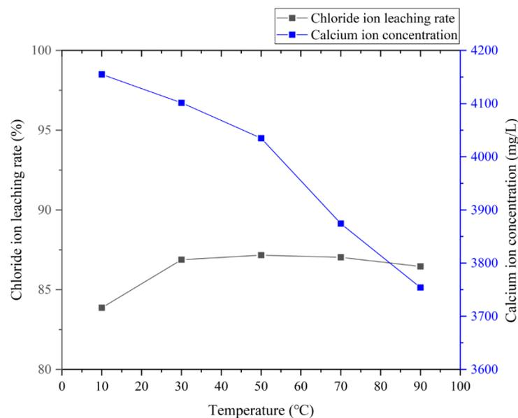
**Figure 5.** Effect of leaching temperature on leaching efficiency of chloride and calcium ions.
