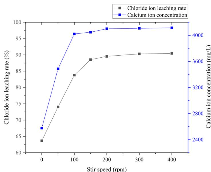
**Figure 4.** Effect of stirring speed on leaching efficiency of chloride and calcium ions.
