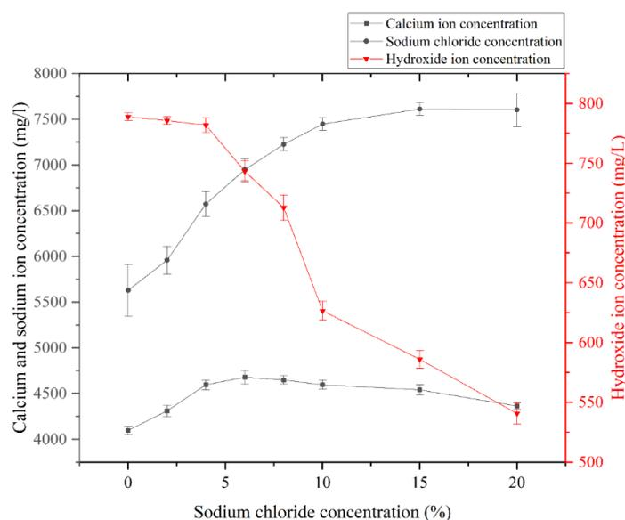
**Figure 9.** Effect of different concentrations of NaCl solution as leaching solvent on the leaching of hydroxide ions, sulfate ions, and calcium ions.
