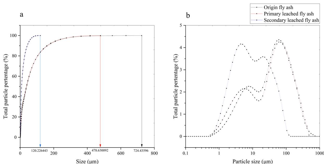
**Figure 14.** Particle size of the fly ash: (a) the integral of the available particle size range and the size at which 100% of the fly ash from the different batches is reached; (b) the logarithmic graph of the different batches of fly ash and the specific size distribution of the fly ash.
