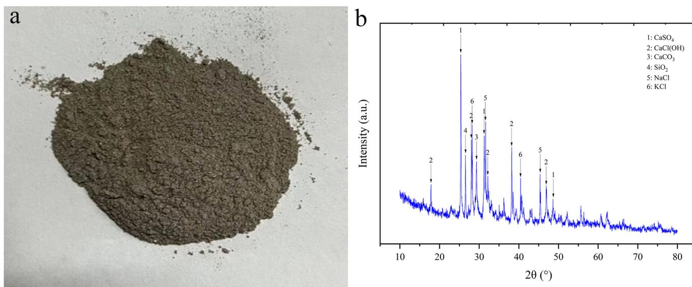
**Figure 1.** Original fly ash (a) brownish-black dry powder; (b) XRD plot.
