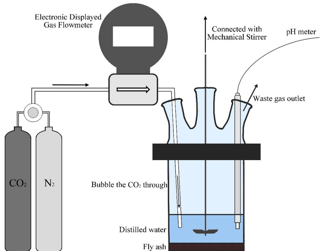
**Figure 2.** Experimental setup for carbonate-assisted leaching.
