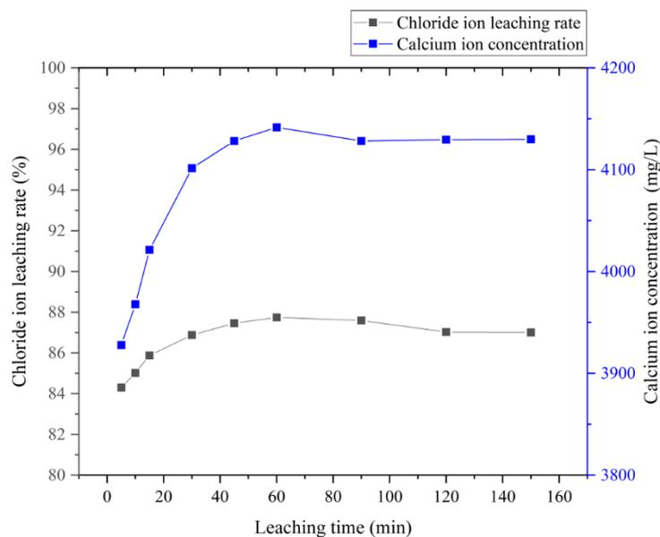
**Figure 3.** Effect of leaching time on leaching efficiency of chloride and calcium ions.
