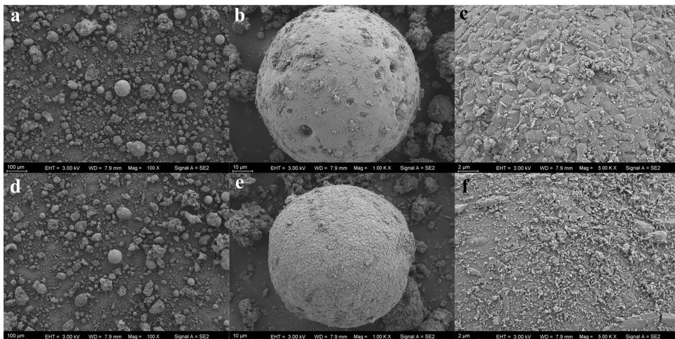
**Figure 7.** SEM images comparing fly ash before and after primary leaching. (a) Before leaching (100  $\mu\text{m}$ ). (b) Before leaching (10  $\mu\text{m}$ ). (c) Before leaching (2  $\mu\text{m}$ ). (d) After leaching (100  $\mu\text{m}$ ). (e) After leaching (10  $\mu\text{m}$ ). (f) After leaching (2  $\mu\text{m}$ ).
