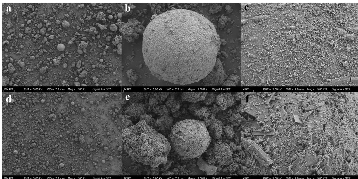
**Figure 12.** Comparison of SEM images of fly ash after primary leaching and after carbonate-assisted leaching. (a) After primary leaching (100  $\mu\text{m}$ ). (b) After primary leaching (10  $\mu\text{m}$ ). (c) After primary leaching (2  $\mu\text{m}$ ). (d) After carbonate-assisted leaching (100  $\mu\text{m}$ ). (e) After carbonate-assisted leaching (10  $\mu\text{m}$ ). (f) After carbonate-assisted leaching (2  $\mu\text{m}$ ).
