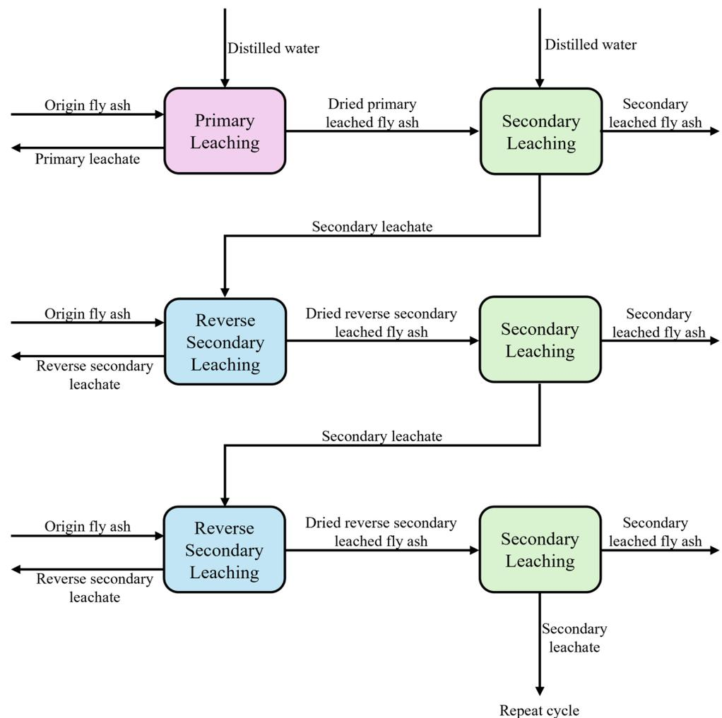
**Figure 8.** Secondary and inverse secondary industrial cycles.
