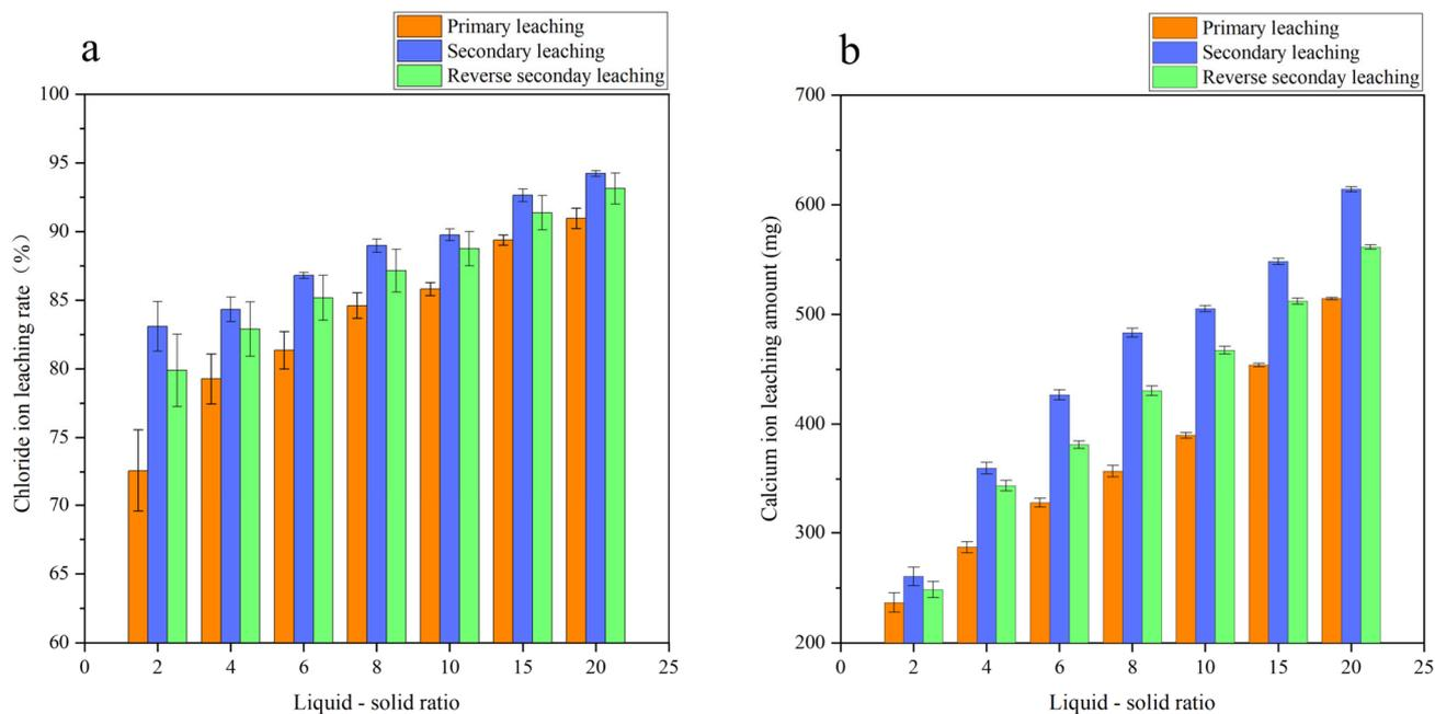
**Figure 6.** Effect of L/S ratio on leaching efficiency of (a) chloride ion; (b) calcium ions.
