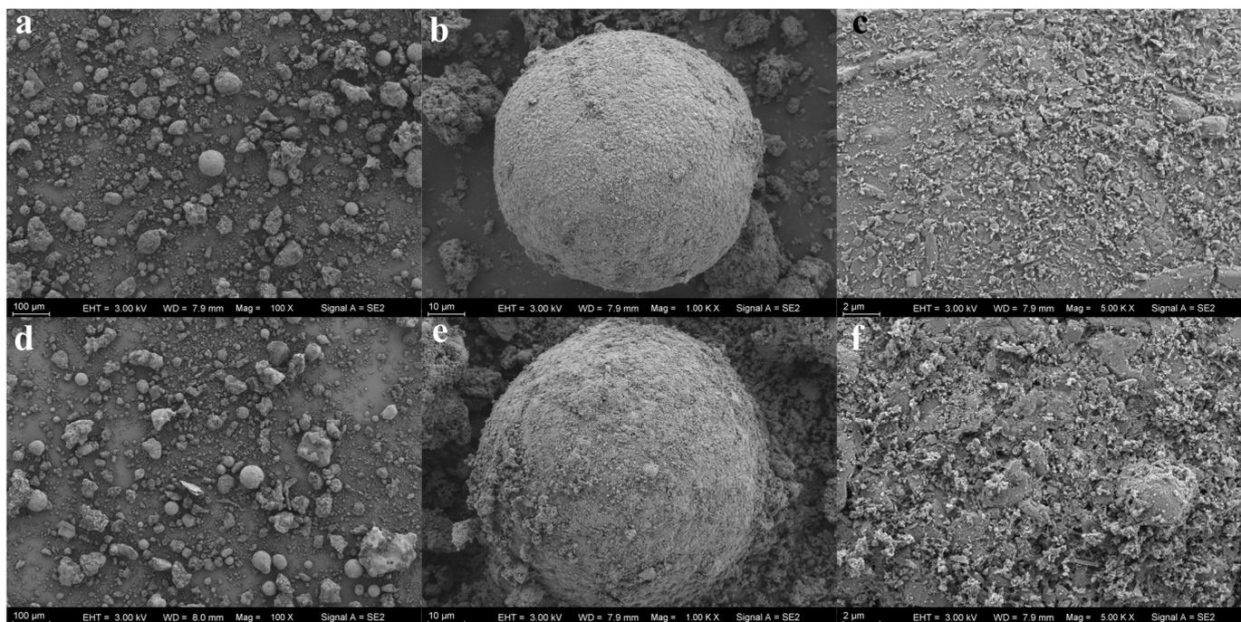
**Figure 13.** SEM images comparing fly ash after primary leaching and ultrasound-assisted leaching: (a) primary leaching (100  $\mu\text{m}$ ); (b) primary leaching (10  $\mu\text{m}$ ); (c) primary leaching (2  $\mu\text{m}$ ); (d) ultrasound-assisted leaching (100  $\mu\text{m}$ ); (e) ultrasound-assisted leaching (10  $\mu\text{m}$ ); (f) ultrasound-assisted leaching (2  $\mu\text{m}$ ).
