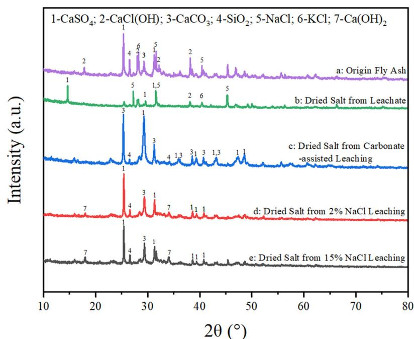
**Figure 10.** (a) XRD plots of (a) original fly ash; (b) dried salts from leachate; (c) carbonate-assisted leachate salts; (d) salts from low (2%) NaCl leach; (e) salts from high (15%) NaCl leach.
