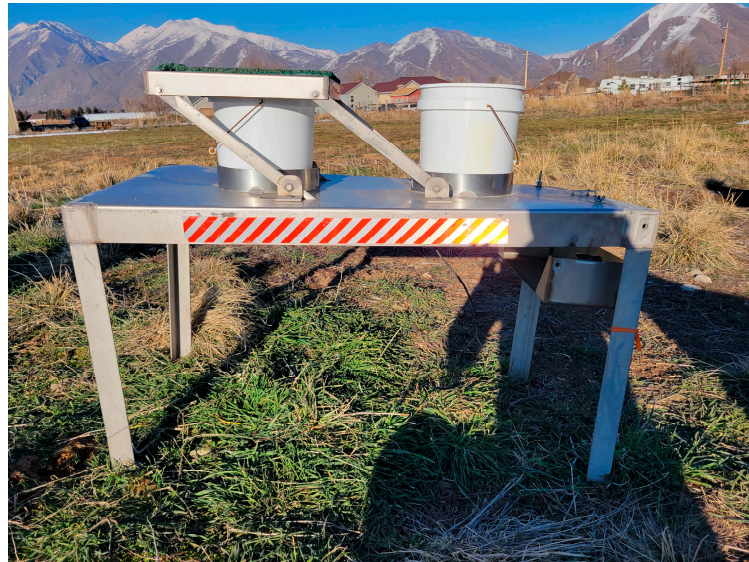
Figure 1. Atmospheric deposition samplers designed to collect wet and dry deposition in separate buckets with a moving lid mechanism.
