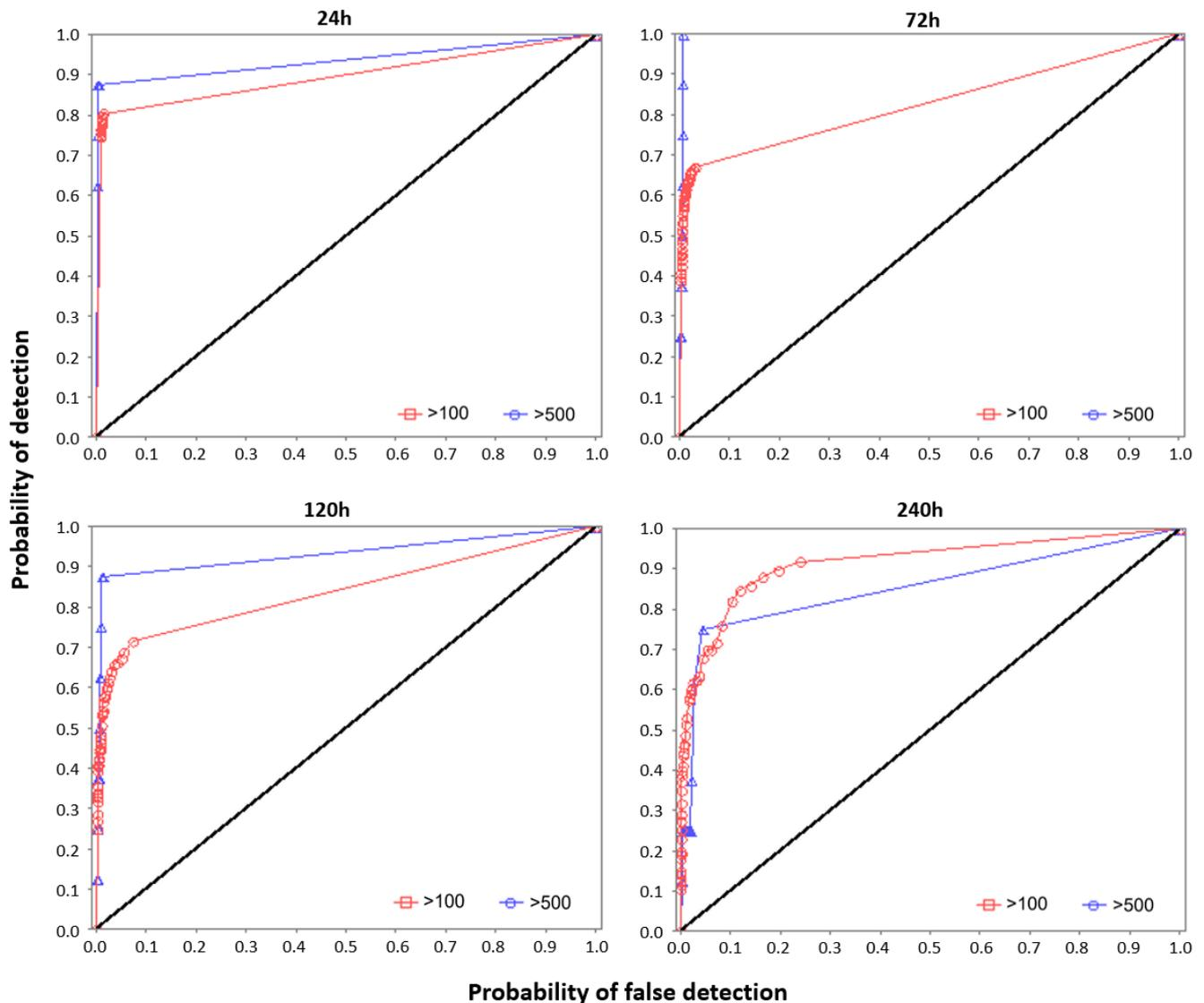
Figure 9. ROC of ensemble inflow forecasts for the forecast horizons of 24 h, 72 h, 120 h and 240 h.
