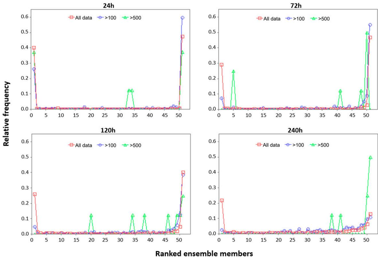
**Figure 8.** Rank Histograms of ensemble inflow forecasts for the forecast horizons of 24 h, 72 h, 120 h and 240 h.
