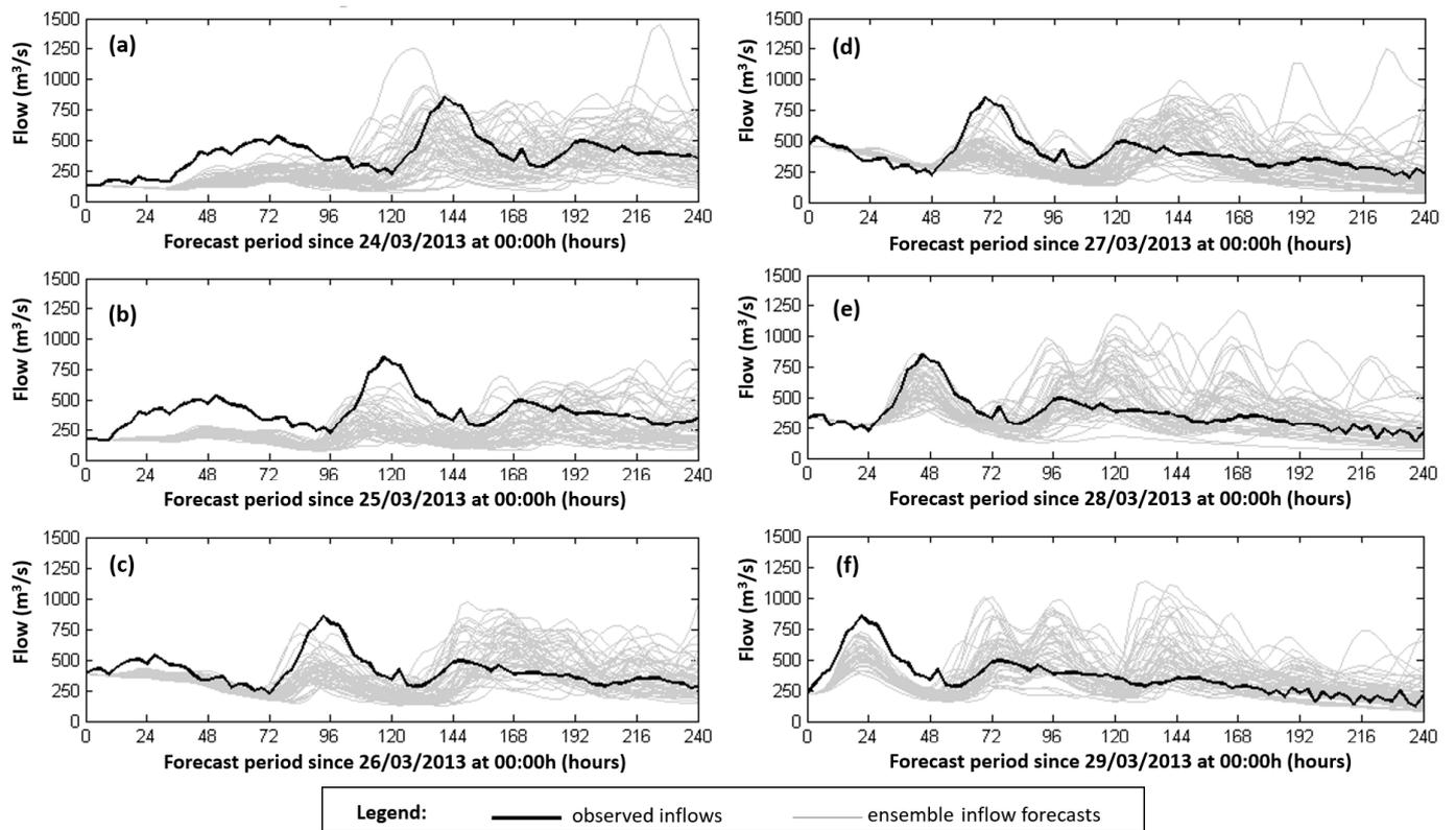
**Figure 2.** Comparison of the ensemble inflow forecasts to the Agueira dam, in the 6 days before to the flood that occurred on 30 March 2013, with the corresponding observed inflows.
