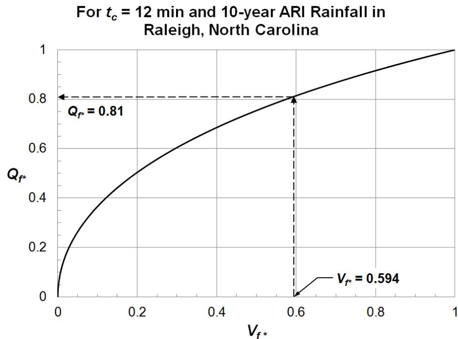
**Figure 7.** Graphical solution of  $Q_{f^*}$  for a catchment with  $t_c = 12$  min in Raleigh, North Carolina.
