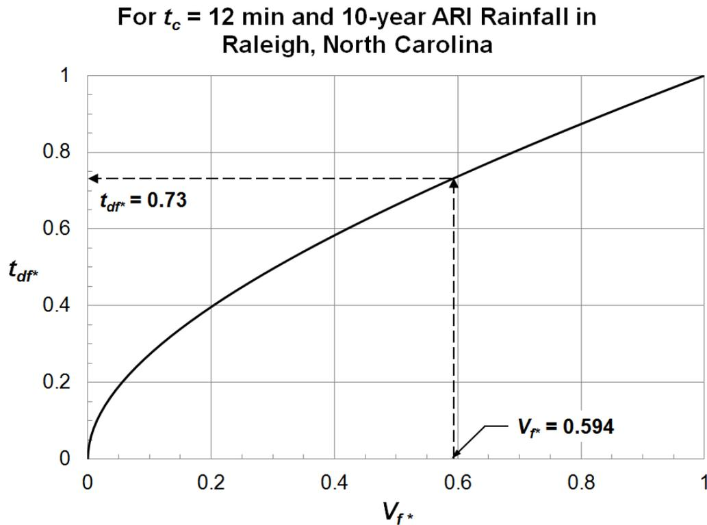
**Figure 6.** Graphical solution of  $t_{df^*}$  for a catchment with  $t_c = 12$  min in Raleigh, North Carolina.
