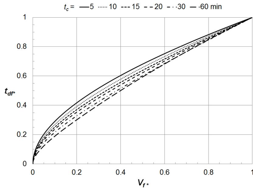
**Figure 4.** Normalized first flush storm duration as a function of normalized first flush capture volume for several values of time of concentration for the semi-arid Southwestern United States covered by NOAA Atlas 14, Volume 1.
