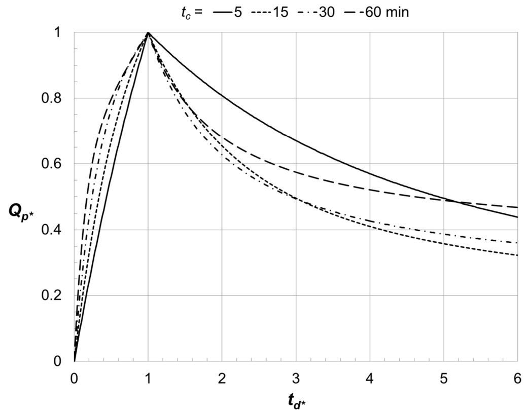
**Figure 2.** Normalized peak runoff rate as a function of normalized storm duration for several values of time of concentration.
