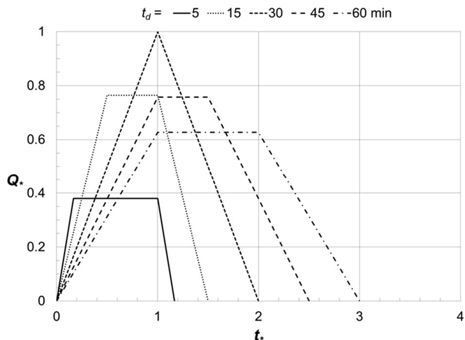
**Figure 1.** Runoff hydrographs from a small catchment given through the modified rational method show the effect of storm duration on peak flow rates and hydrograph shape.
