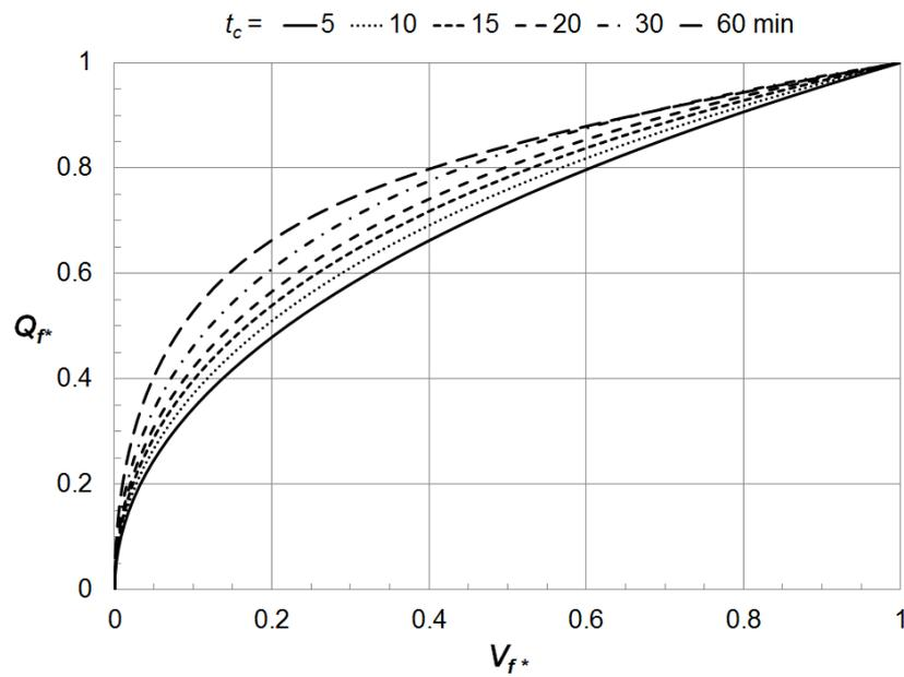
**Figure 3.** Normalized first flush design flow rate as a function of normalized first flush capture volume for several values of time of concentration for the semi-arid Southwestern United States covered by NOAA Atlas 14, Volume 1.
