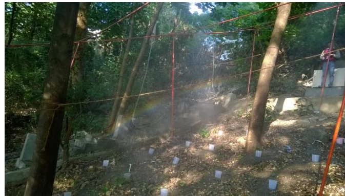
Figure 4. Rainfall experiment for calculation of coefficient of uniformity.
