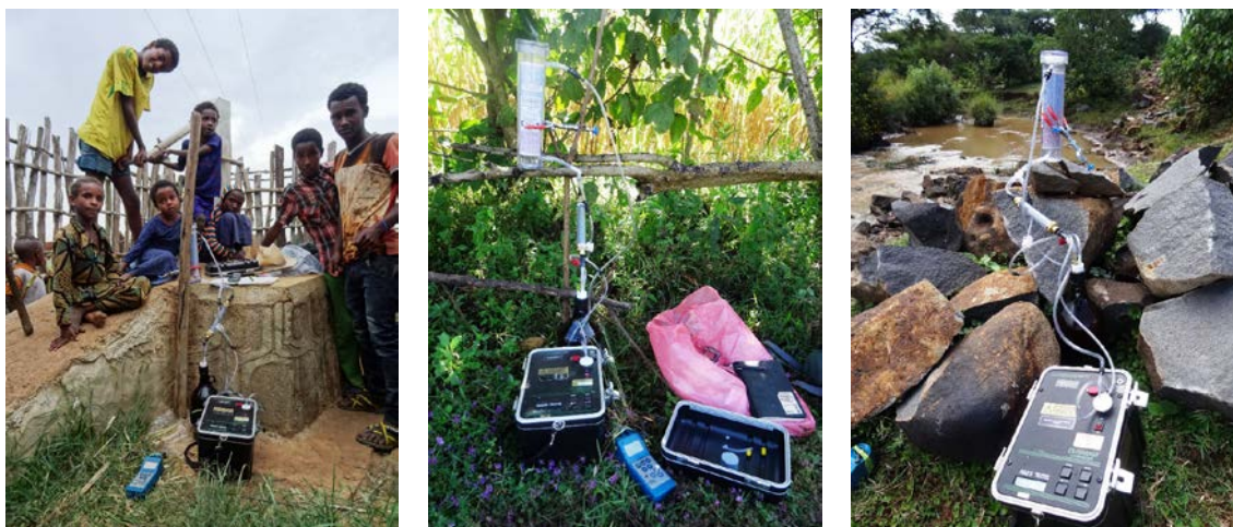
Figure S-1. Photographs showing radon-222 testing. The in-situ EC, pH, and temperature meter is also visible.
