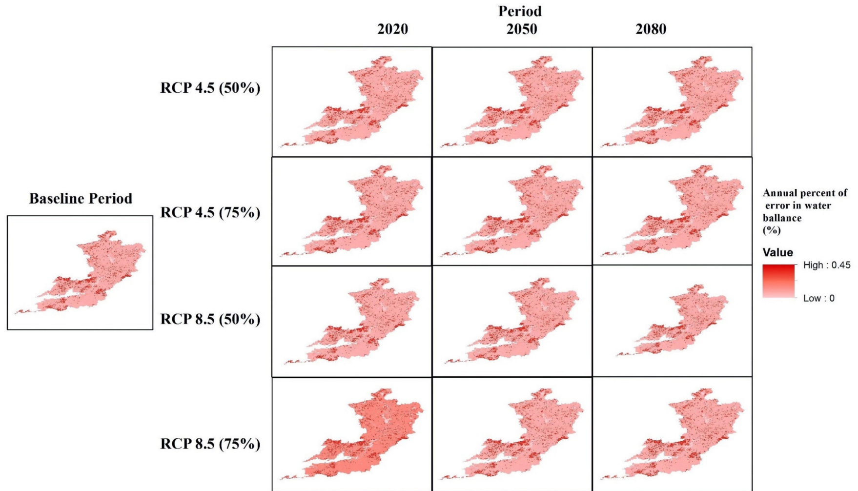
Figure A12. The spatially distributed average annual error/change in storage in water balance (mm/year) for each climatic period and land use scenario simulated by GEO-CWB.
