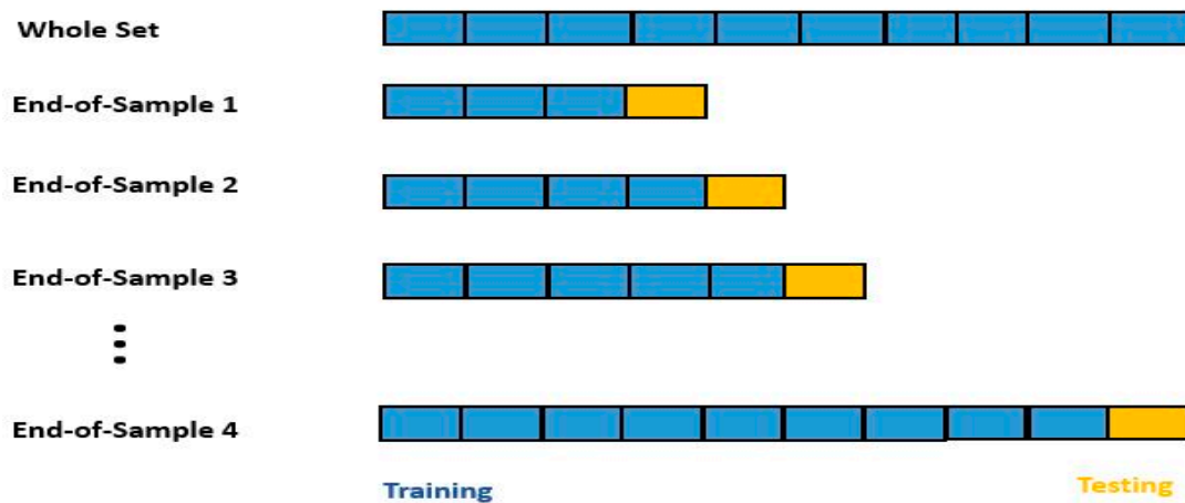
Figure 7. Diagram of the time series 4-sliding window validation method. Adapted from LaBarr (2018).
