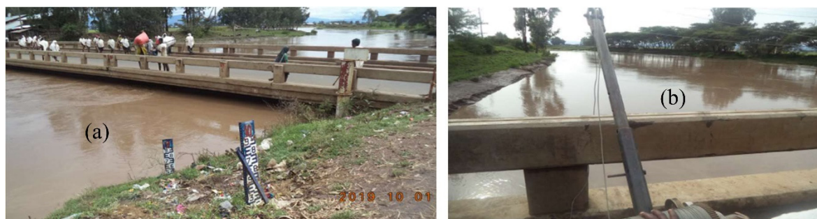
Figure 2. Rivers at full stage: (a) Submerged gauging staff by sediment depositions at Ribb near Addis Zemen station (2019), (b) Flow measurements on Ribb at Addis Zemen using crane over the bridge during peak flows (2016).
