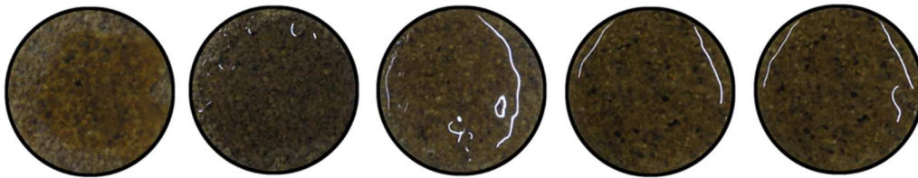
Figure 9. Example of snapshots of the window of coarse sand specimens once the test stopped with no fractures being induced in coarse bio-cemented sands across various cementation levels.
