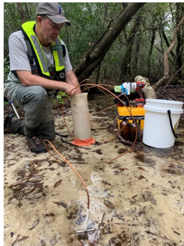
Figure 5. Upwelling groundwater from 1 to 1.2 m below the creek in the upper part of the sand and gravel aquifer was sampled using a peristaltic pump (yellow case) attached to the temporary well (foreground). A 6.35 mm inner diameter copper tubing and a vitex tube were used to collect the samples. The graduated nylon cylinder was used for the collection of dissolved gas samples and to house the sonde during measurements of physical properties and chemical constituents of groundwater. [Photograph by James E. Landmeyer, U.S. Geological Survey].
