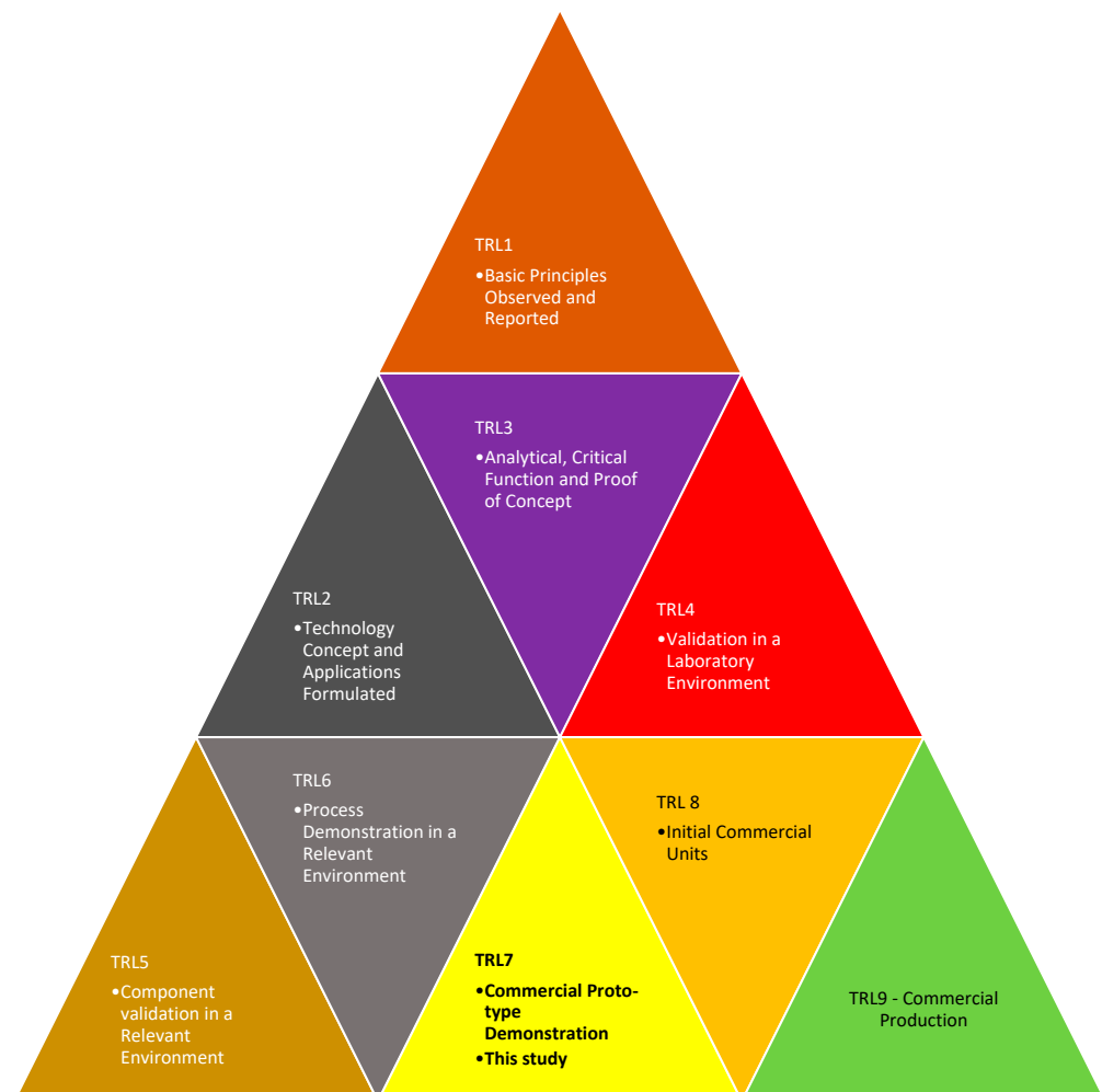
Figure A4. Technology readiness levels associated with zero-valent iron desalination research in diffusion reactors. This study is an initial TRL7 demonstration of a batch flow, bubble column, static bed, diffusion reactor operation (Figure A3). Patents [US9624113B2; US9828258B2; US2018/0009678A] have demonstrated a TRL7 operation for a batch flow, emulsified bubble column, fluidised bed reactor (Figure A3). It is possible that unpublished TRL7 demonstrations have been undertaken for a continuous flow, contact flow, fluidised bed reactor (Figure A3) and a continuous flow, fluidised bed, recirculating reactor (Figure A3).
