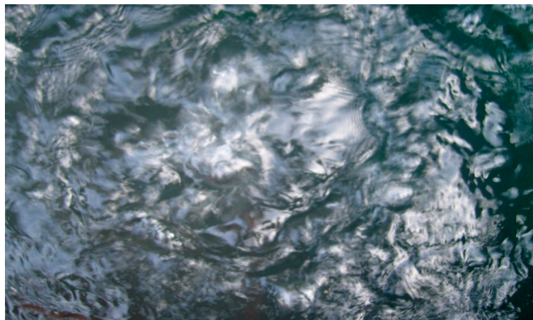
Figure 14. Reactor in operation. View of the air–water contact, showing a turbulent environment. Field of view = 25 cm.
