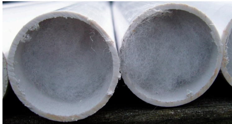
Figure 3. Example of open-ended ZVI cartridges prior to being placed in a reactor train. The entrance to the cartridge is filled with filter wool.
