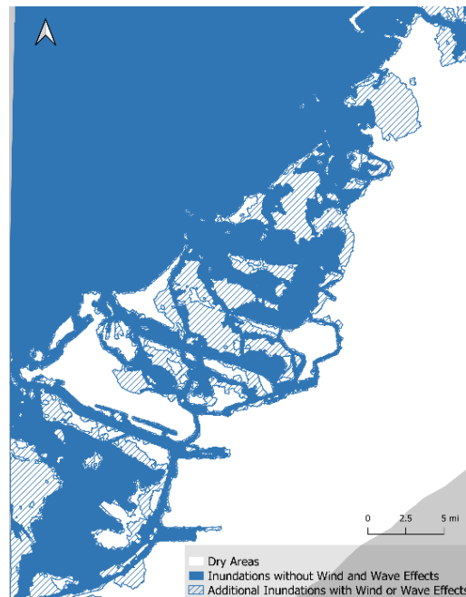
Figure 6. Predicted inundation extent for the Abu Dhabi area—SLR with tidal effect only, with and without the effect of winds or waves.
