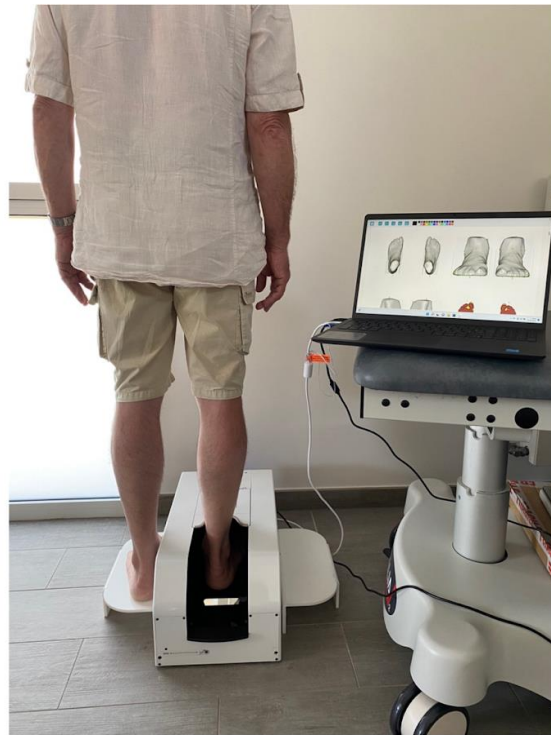
Figure 1. Subjects were scanned in a standing position (one foot in the scanner, the other one on a footrest at the same height).
