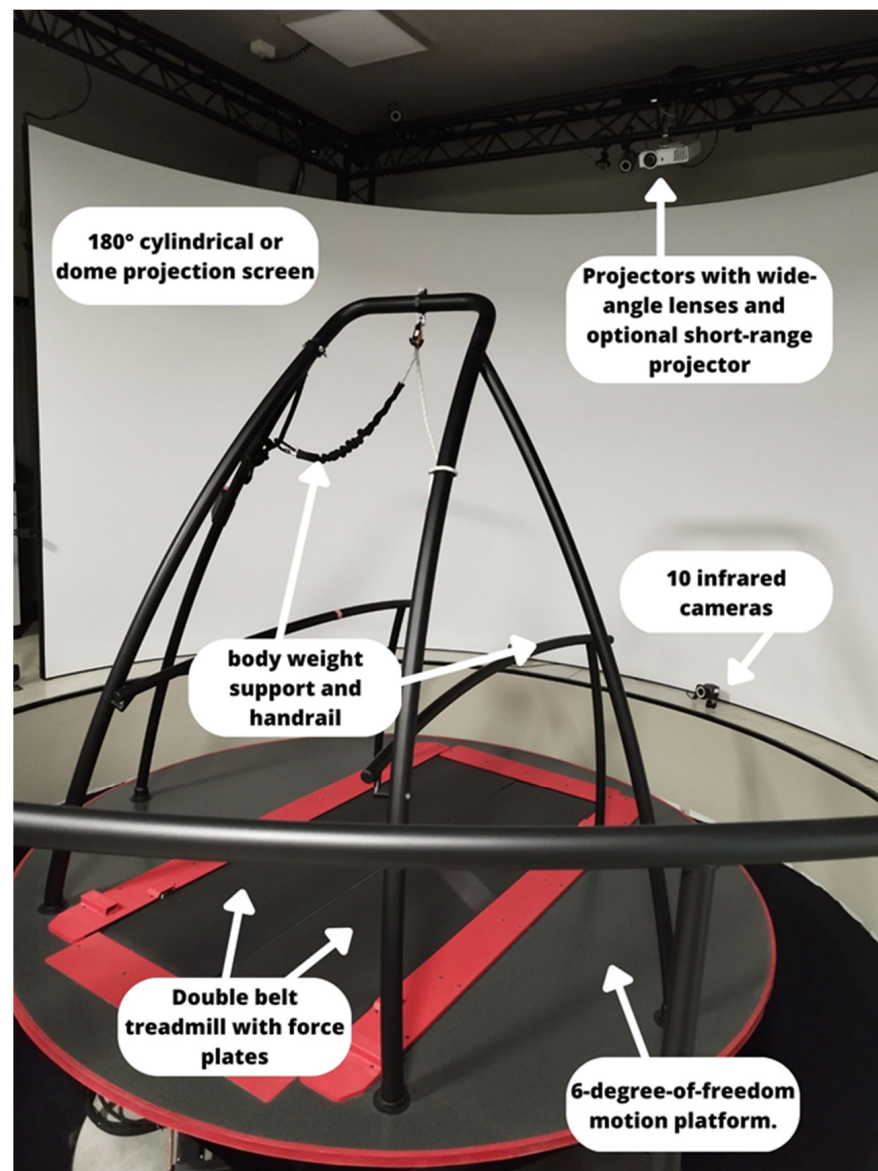
Figure 4. The CAREN EXTENDED system and its components, allocated at the IRCCS Neurolesi Center “Bonino-Pulejo”.
