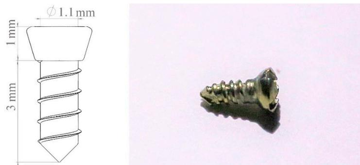
**Figure 5.** The size and shape of the self-taped implant. The diameter of the implant was 1.1 mm, with a total length of 4 mm and a transmucosal length of 1 mm.
