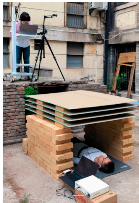
Figure 12. Experimental outdoor obstructed detection scenario for extracting contact and non-contact human life signals.
