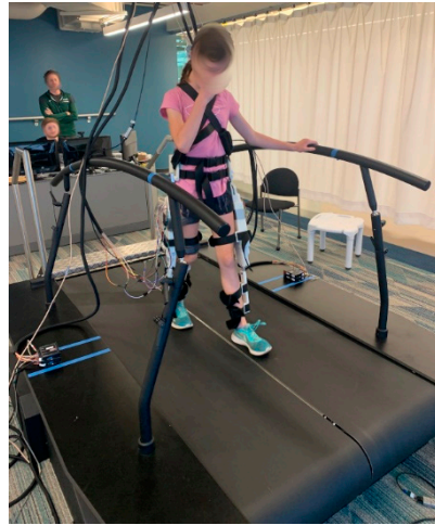
Figure 3. Experimental setup on the instrumented treadmill with the volunteer subject wearing the pediatric exoskeleton.
