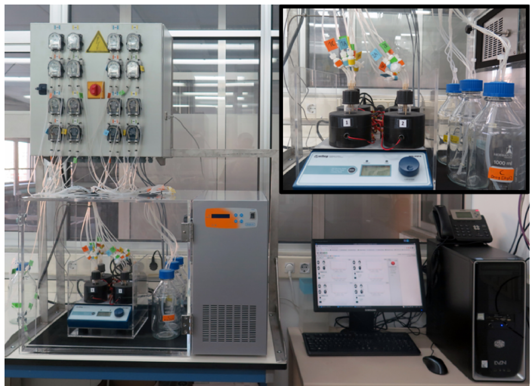
Figure A1. Photography illustrating the morbidostat setup, including the fluidic system, the incubator, the control box, and the associated desktop computer.
