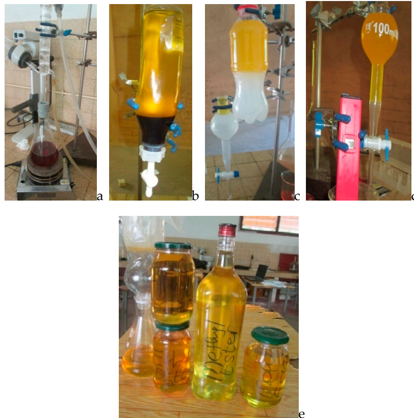
Figure 1. Biodiesel production process: (a) production, (b) separation, (c) and (d) washing, and (e) final products.
